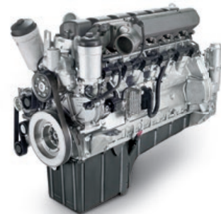
Series 460 A true trooper in all conditions, delivering proven performance with an evolved design. 220–375 kW (295–503 bhp)
